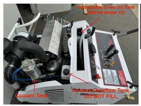
Alternate view of the coolant, coolant overflow, and hydrostatic drive oil tanks.
