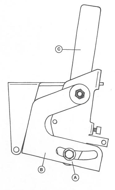
Needle valves wear over time. To adjust the valve to keep it from dropping, loosen the 5/16" bolt and nut (A) with two half inch wrenches. Rotate the arm (B) forward slightly, and re-tighten (A).
